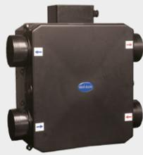
The Integra Heat Recovery unit has been specially designed to provide ventilation for smaller residential or commercial applications up to 180m<sup>2</sup>. With low power consumption, this simple ducted heat recover system has been specially designed to extract heat energy from the outgoing air and transfers this energy to the incoming fresh air tempering it, without the two air streams mixing.
