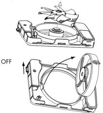
Clean the duct/pipe if there is any dirt present inside. Failure to do this may result in a risk of impaired capacity.
