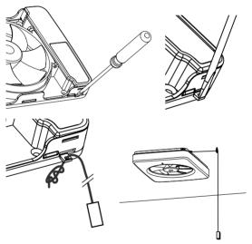
Once installation is complete, push the safety switch down to position I – ON, to make the fan active again.
