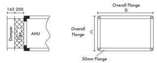
Dampers are supplied with extended spindles - suitable for motorisation as standard.
