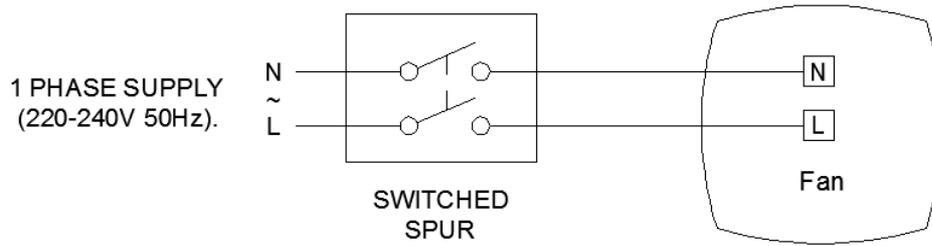
**Fig.2** Continuous boost 1 with no trickle facility. (The fan is internally fused)
