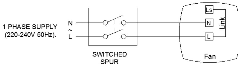
**Fig.3.** Continuous trickle with boost facility. (The fan is internally fused)
