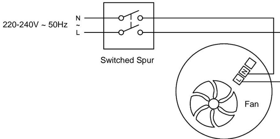
**Fig.2** Continuous boost with no trickle facility. (The fan is internally fused)
