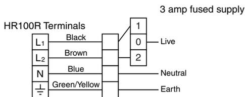
**NOTE:** Wiring must be via a 3A fused switched spur with a 3mm contact separation in each pole. The wiring should be suitably (BASEC or HAR) approved cable of appropriate current carrying capacity.
