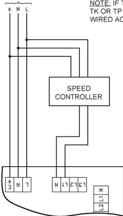
NOTE: IF THE SPEED CONTROLLERS HAVE TK OR TP TERMINALS, A LINK SHOULD BE WIRED ACROSS THESE TERMINALS.
