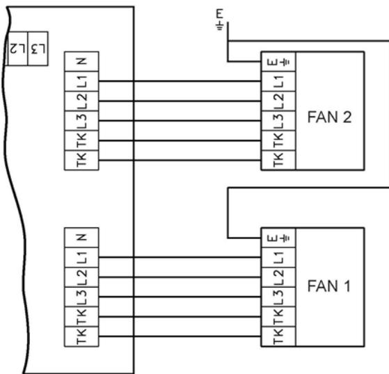
NOTE: 3 PHASE FANS MUST HAVE EXTERNALLY CONNECTED THERMAL OVERLOAD PROTECTION.
