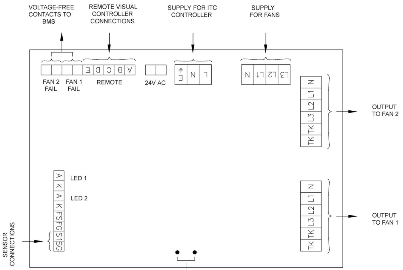
LINK TO SELECT 24HR. CHANGE OVER. MODEL ITC-DS ONLY IS INSERTED HERE
