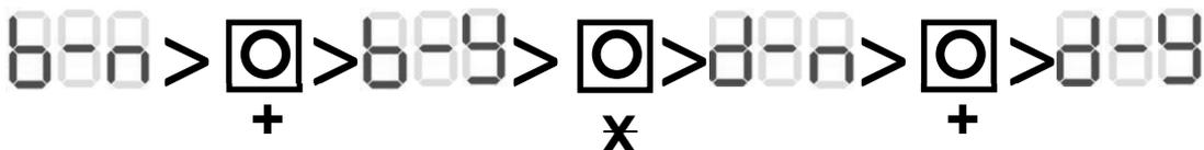
Mode and up buttons pressed to change the setting to Bathroom and ducted modes
