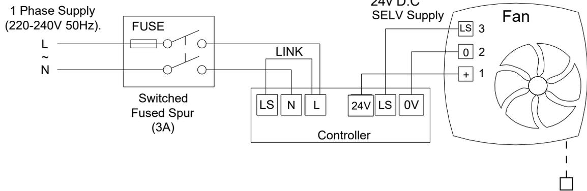
Fig.6 Continuous trickle with boost facility via LS or internal pull-cord, SELV models
