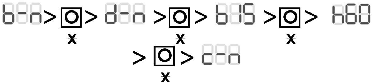
Mode button being pressed to scroll through menu. This set up is for a kitchen, in a through the wall installation with 15 minute boost timer, 60% rH set point and not in comfort mode.
