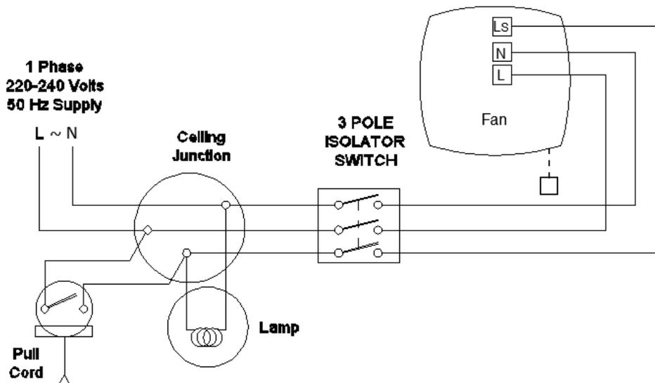
Fig.4 Continuous trickle with pull-cord boost SELV models
