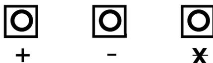
The + button is used to increase the value of a setting, the – button is used to reduce the value of a setting and the X (Mode) button moves to the next setting.
