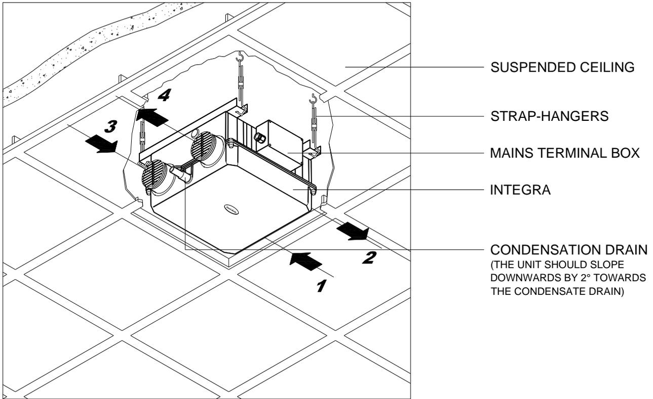
**Fig. 1b. SUSPENDED IN ROOF VOID**
