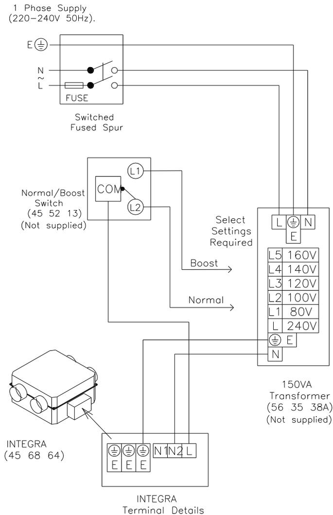
**Fig.2d (Integra controlled via two sensors/switches and a 150VA transformer to give 3 running speeds).**
