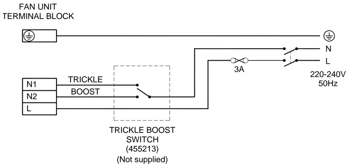
**Fig.2b (Integra operated by an Ambient Response humidity sensor)**
