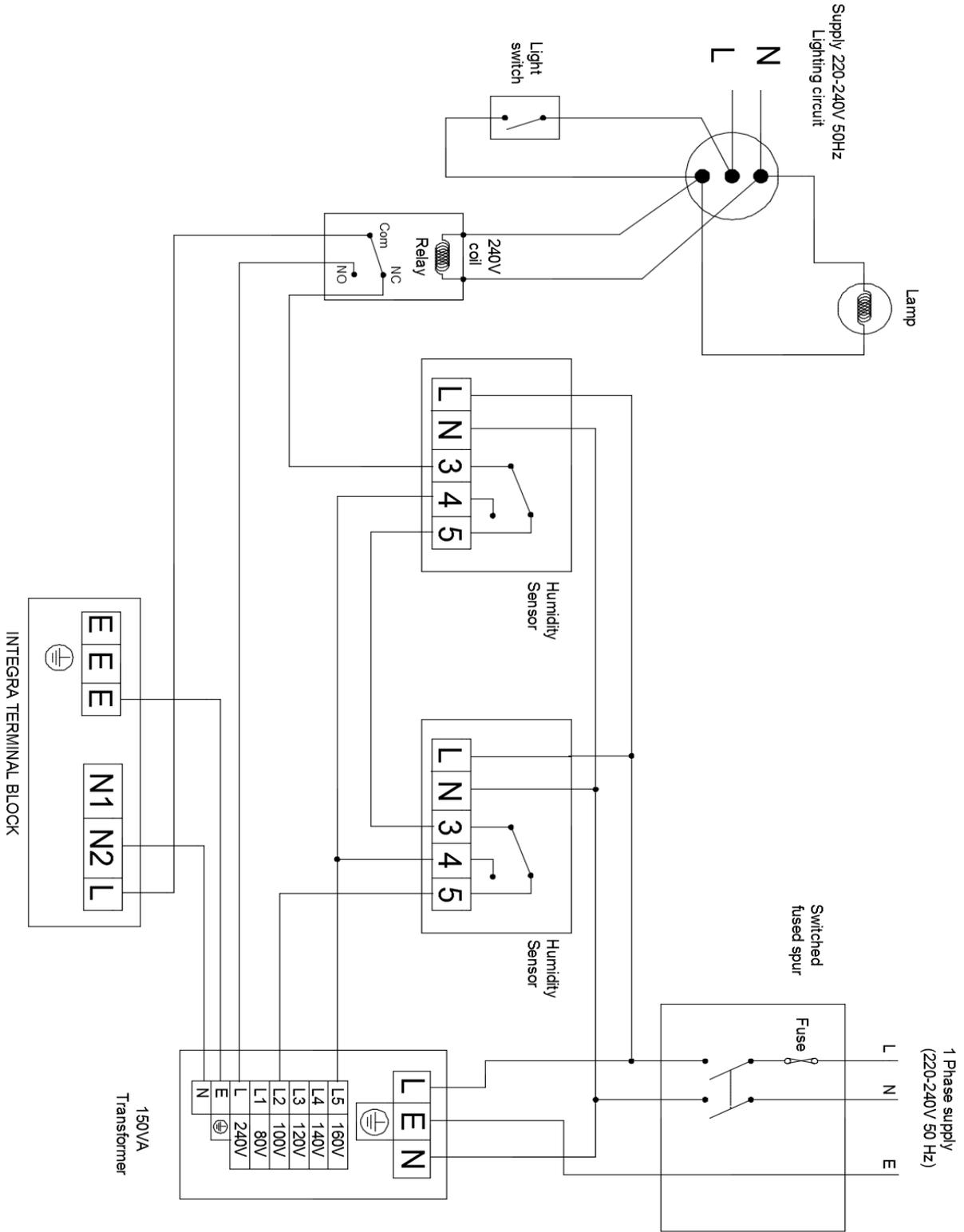
**Fig.3 Summer Bypass/ Extract Only Switch (409999 NOT supplied)**
