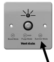
If the LED on the Remote Boost switch flashes green, there is an error with the units Temperature sensor. The sensor is used by the frost protection system. If the unit was in Summer mode it will return to normal operation. Please contact the Vent-Axia Technical Support for assistance.
