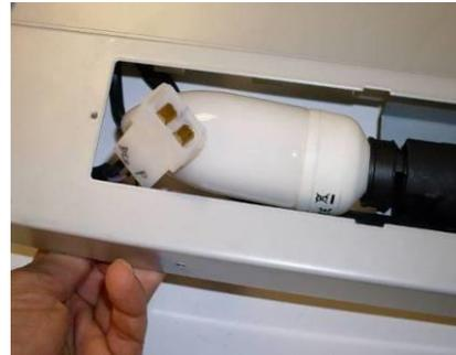
Figure 9: Passing cable through
