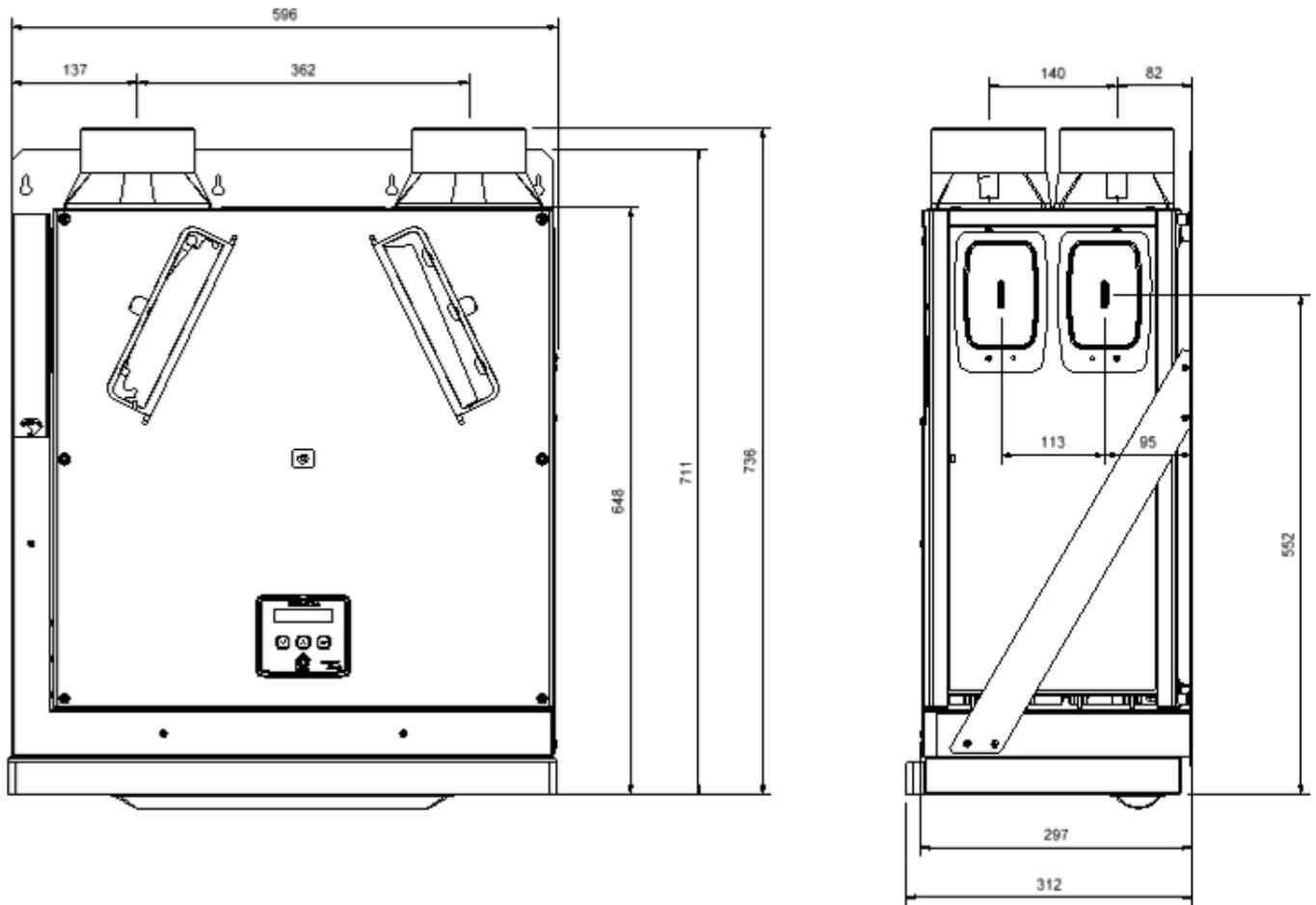
Figure 2: Sentinel Kinetic with Cooker Hood Dimensions
