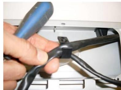
Figure 11: Using cable clip to secure the cable
