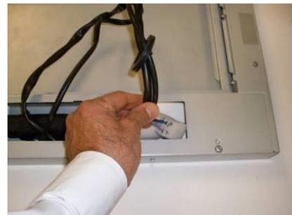
Figure 10: Insert cable opposite direction
