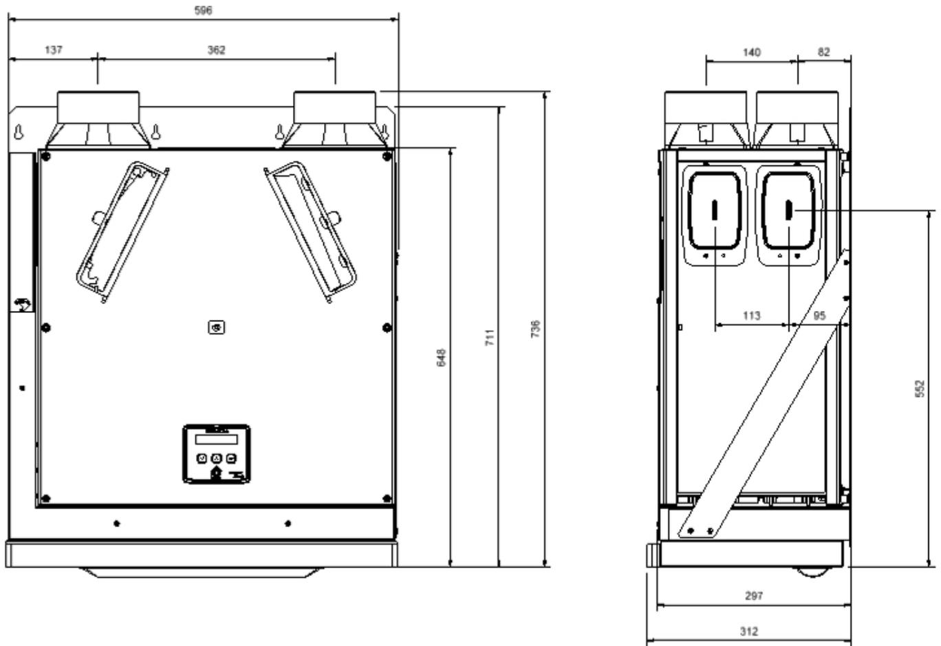
Figure 2: Sentinel Kinetic with Cooker Hood Dimensions
