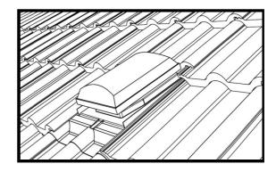
SUITABLE FOR ROOF PITCHES OF BETWEEN 20° AND 60° FOR PITCHES ABOVE OR BELOW THIS CONSULT VENT-AXIA TECHNICAL SUPPORT
