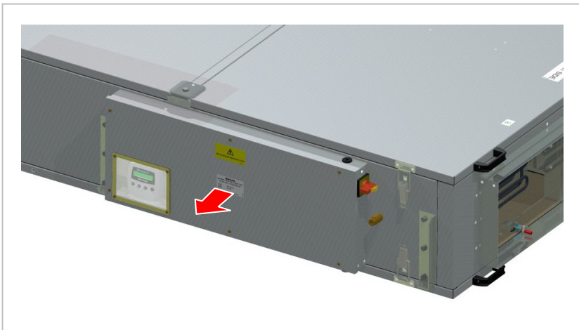
Figure 8: Control Panel Access
