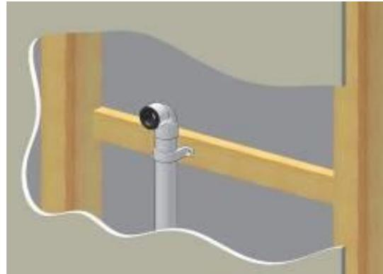
5. Fit the flexible condensate pipe to a 22mm diameter x 280mm long condensate pipe with worm drive clip.
