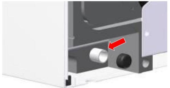
3. If not already fitted, fit the flexible condensate pipe and secure with worm drive clip
