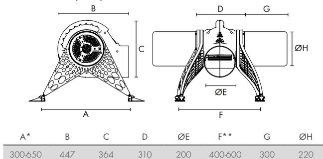
\*Variable to allow for adapting product height. \*\*Variable to adapt to differing joist widths. Height will vary as A dimension changes
