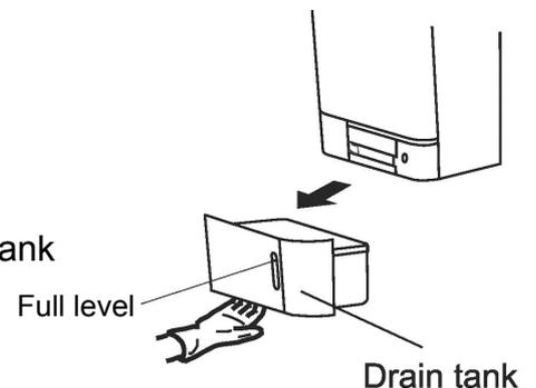
Open the drain tank cover and empty out the water.
