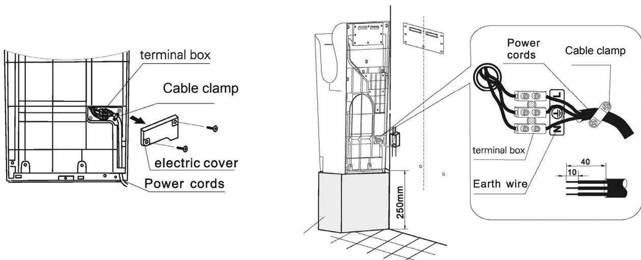
Fit terminal block cover to rear of dryer
