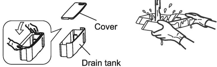
At regular intervals (at least once a week) carefully pour 200cc (around a cup) of water through the drain hole. (to prevent it from getting clogged up).
