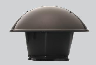
The Unitex Roof Cowl System greatly simplifies the roof termination of mechanical ventilation systems. Consisting of an attractive epoxy finished cowl with a lead weather slate and a range of direct connection reducing fittings. It is suitable for connection to spiral duct, soil pipe and flexible duct from 125 to 250mm diameter.
