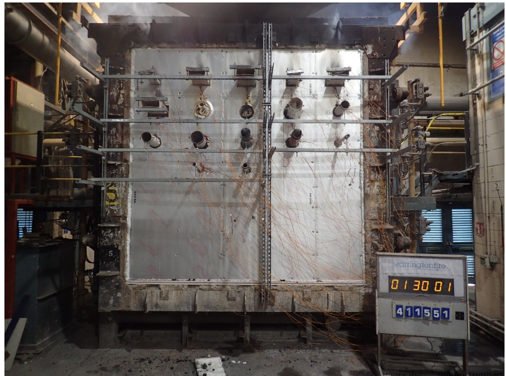
The unexposed face of the test construction after a test duration of 90 minutes
