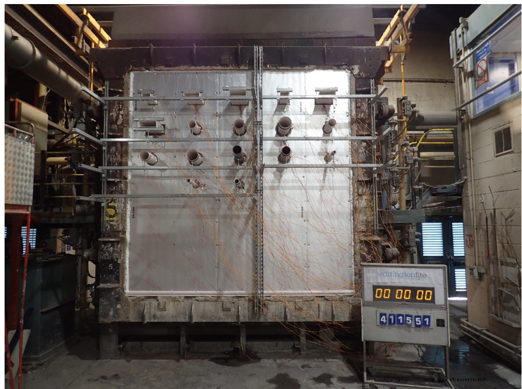
The unexposed face of the test construction prior to the start of the test
