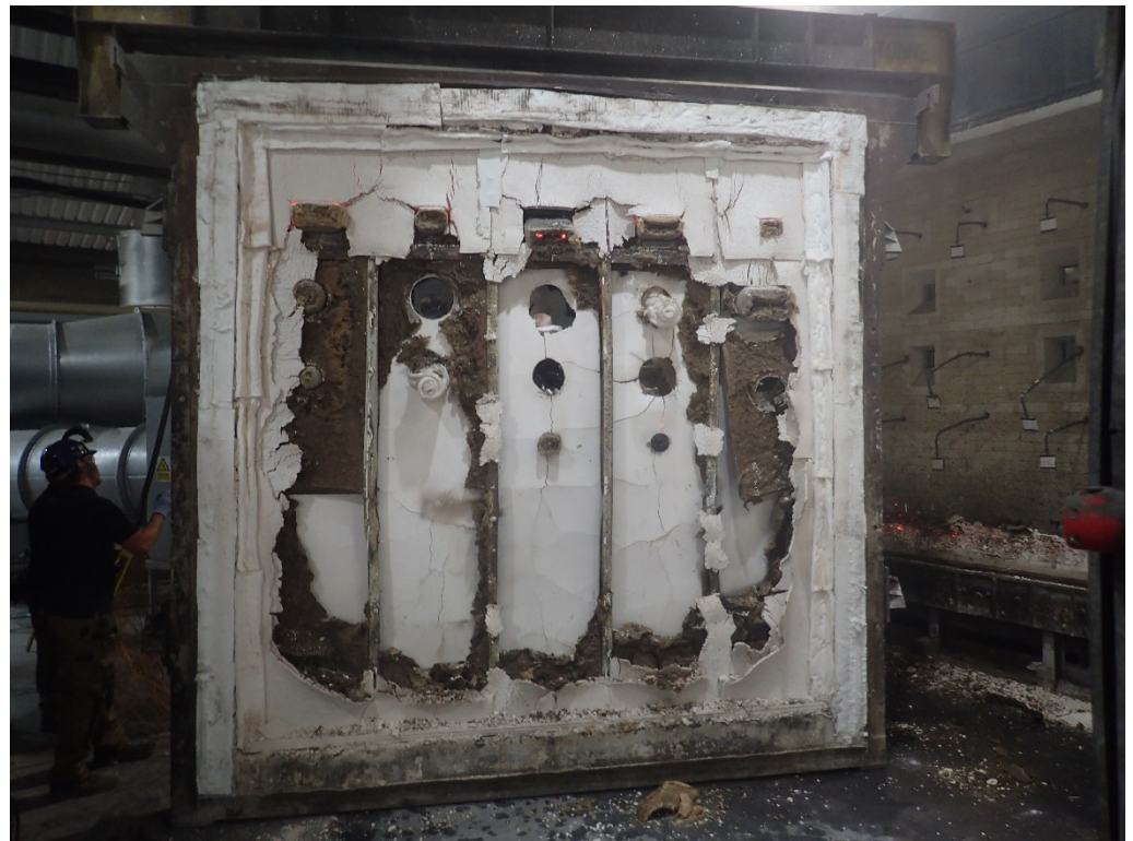
The exposed face of the test construction after the test
