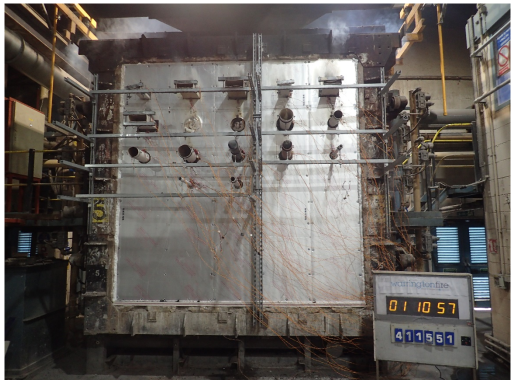
The unexposed face of the test construction after a test duration of 70 minutes
