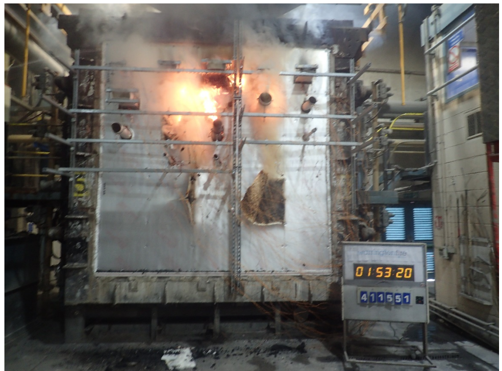
The unexposed face of the test construction after a test duration of 113 minutes
