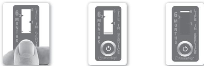
1. Activation: Fully squeeze the activation button between thumb and finger. A red line will appear within 1-2 minutes to show that the Timestrip has been activated.
