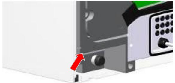
2. Remove the black Cap from the end of the condensate stub at the rear of the unit.
