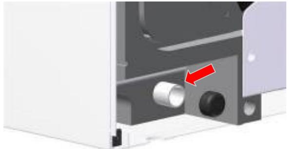
3. Fit the vertical condensate pipe and secure with worm drive clip
