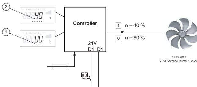
1 Setting “Set Intern1” (depending on device type in: %, Hz, rpm)
