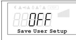
The individually made device configurations (User Settings) can be saved and, with the corresponding PIN input (9091), can be reestablished.
