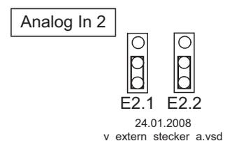
**External Setpoint** via external signal instead of “Setpoint 1”. The “external Setpoint” function must be activated in base setup **[1E]** for “E2 function”. The active external Setpoint value is displayed in the “info” menu group.
