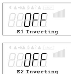
Factory setting for Inverting inputs = “OFF” (if input activated) (signal: 0 - 10 V, 0 - 20 mA, 4 - 20 mA).
