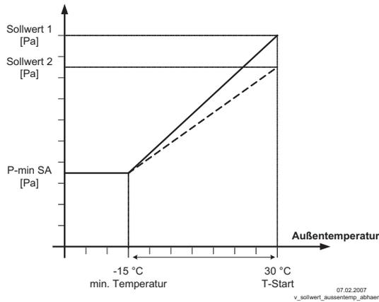
An outside temperature compensation can be activated (sensor connection “E2” = “Analog In 2”) when being operated as a pressure regulation device.
