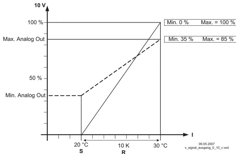
Example: Setpoint ventilation 25.0°C, Offset -5.0 K, Pband 10.0 K
