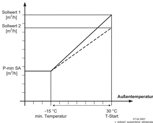
An outside temperature compensation can be activated (sensor connection “E2” to “Analog In 2”) when being operated as a air volume regulation device.
