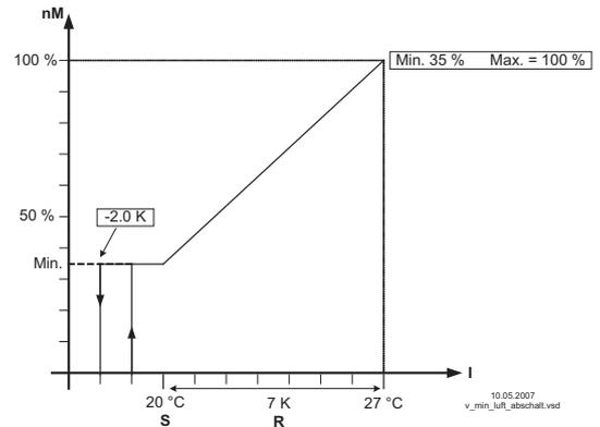
Minimum speed cut off (idealized principle diagram)
