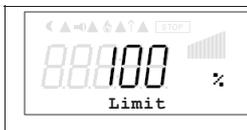
After allocation of a digital input (☞ IO Setup) an adjustable limitation of the modulation can be activated via a digital input (“D1”, “D2”, ..).
