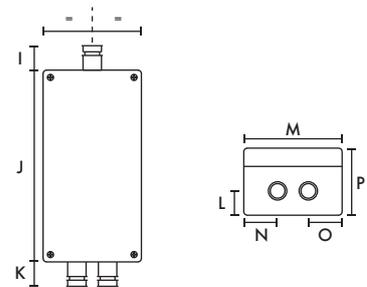
The LTG is an air temperature sensitive speed controller, which can be set between 20°C and 50°C. The controller is suitable for controlling up to 5 MX units when used in conjunction with a VG31 Multi Unit Controller.
