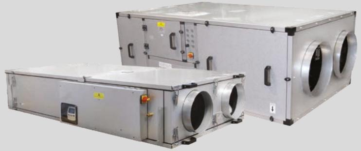
Mini and Midi Models are manufactured with a frameless construction from single skinned Aluzinc panels, internally lined with 90kg/m<sup>3</sup> high efficiency acoustic and thermally insulating foam (fire retardant to BS476 Part 7 Class 1 & Part 6 Class O). Aluzinc panels allow for all units to be mounted either internally or externally as standard (IPX4). An optional inlet cowl is available for roof mounting applications if required.
