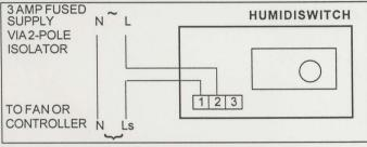
Connect to 2 and 1 for switch to operate on rise in humidity.
