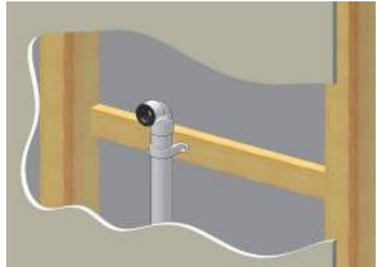
5. Fit the 180 degree bend supplied to a 22mm diameter x 280mm long condensate pipe with worm drive clip.
