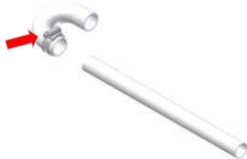
6. Fit pipe assembly into waste pipe and secure 90 deg elbow to condensate spigot with worm drive clip.
