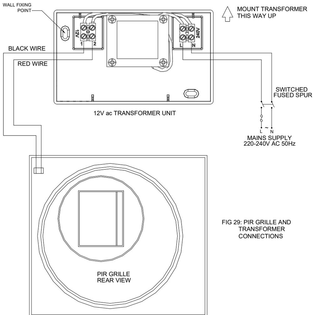
FIG 29: PIR GRILLE AND TRANSFORMER CONNECTIONS
