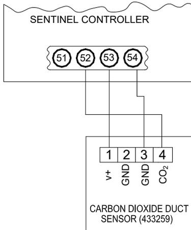
FIG 19: CARBON DIOXIDE DUCT SENSOR CONNECTION TO SENTINEL CONTROLLER
