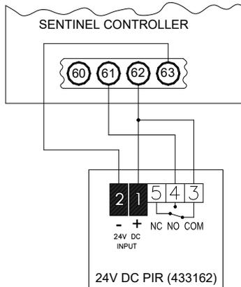
FIG 16: PIR MASTER ENABLE CONNECTION TO SENTINEL CONTROLLER (NOTE! ENSURE CONTROLLER LINK 61 to 62 IS REMOVED BEFORE CONNECTING PIR)
