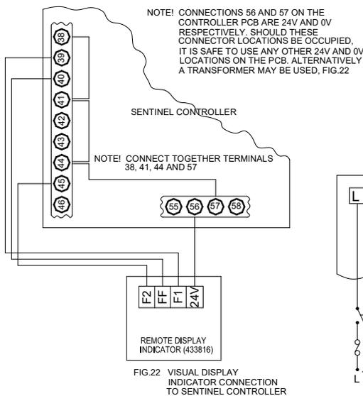
FIG 22 VISUAL DISPLAY INDICATOR CONNECTION TO SENTINEL CONTROLLER
