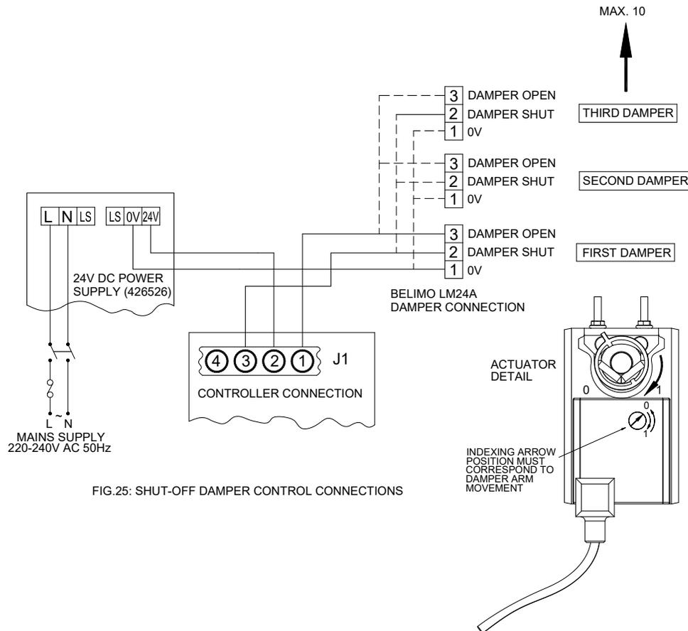
FIG.25: SHUT-OFF DAMPER CONTROL CONNECTIONS
