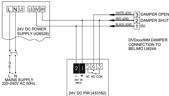
FIG 27A: DUCT DAMPER CONNECTION CIRCUIT TO PIR (TO AMBIENT RESPONSE HUMIDISTAT)
