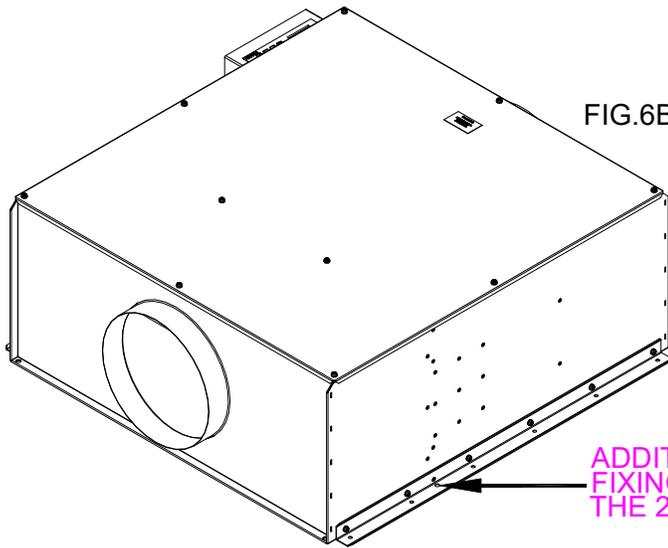
FIG.6B: SUPPORT BRACKET USED ON LARGER SENTINEL TWIN UNITS
