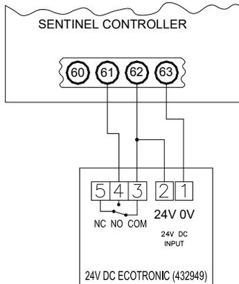
FIG 15: HUMIDISTAT MASTER ENABLE CONNECTION TO SENTINEL CONTROLLER (NOTE! ENSURE LINK 61-62 IS REMOVED)
