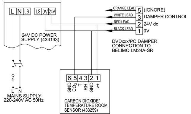
FIG 28B: CARBON DIOXIDE ROOM SENSOR CONNECTION TO PROPORTIONAL DAMPER
