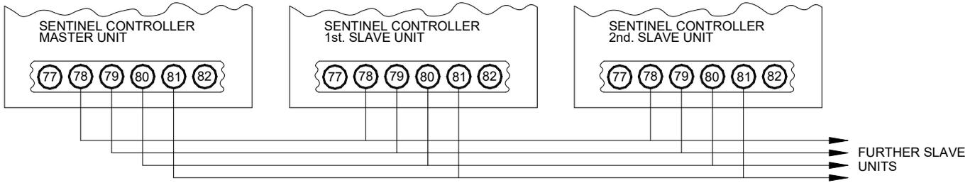
FIG 24: MASTER-SLAVE NETWORK CONNECTIONS
