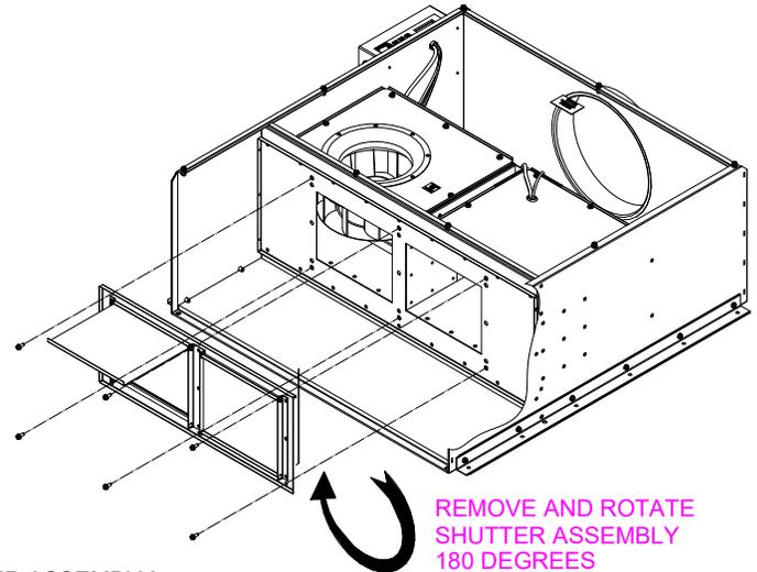
REMOVE AND ROTATE SHUTTER ASSEMBLY 180 DEGREES
