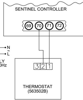
FIG 14: THERMOSTAT CONNECTION DIAGRAM
