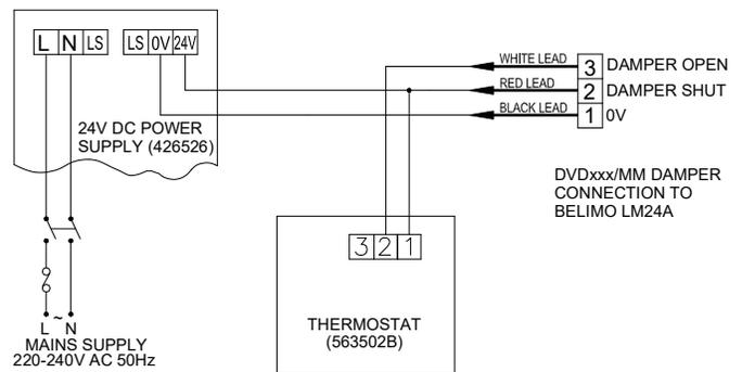
FIG 27D: DUCT DAMPER CONNECTION CIRCUIT TO THERMOSTAT
