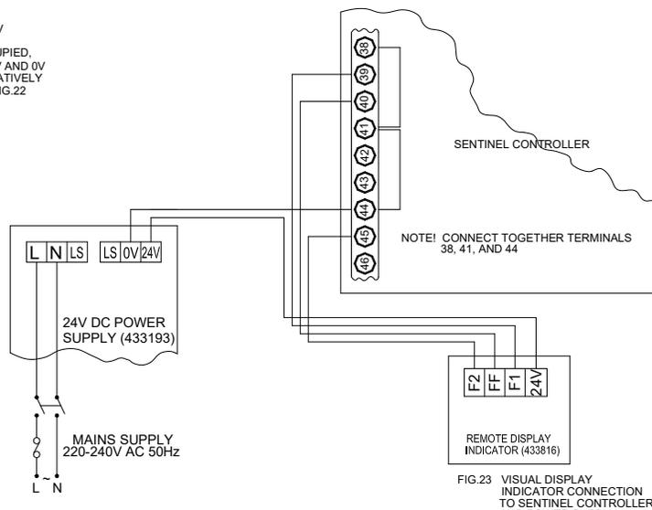
FIG 23 VISUAL DISPLAY INDICATOR CONNECTION TO SENTINEL CONTROLLER AND POWER SUPPLY
