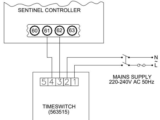
FIG 17: TIMESWITCH MASTER ENABLE CONNECTION TO SENTINEL CONTROLLER (NOTE! ENSURE LINK 61-62 IS REMOVED)
