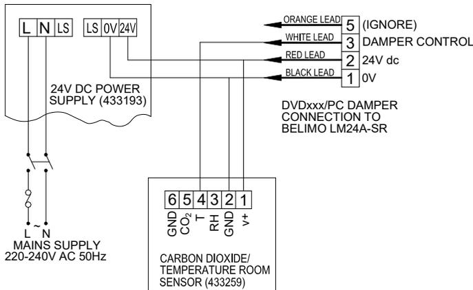
FIG 28C: TEMPERATURE ROOM SENSOR CONNECTION TO PROPORTIONAL DAMPER
