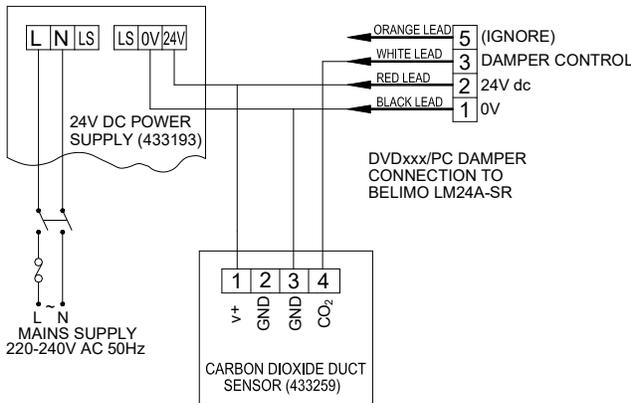
FIG 28A: CARBON DIOXIDE DUCT SENSOR CONNECTION TO PROPORTIONAL DAMPER
