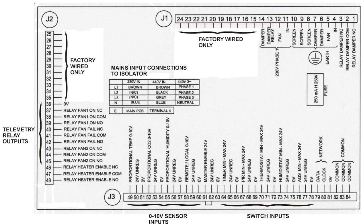
Fig.1 Controller Connections Layout
