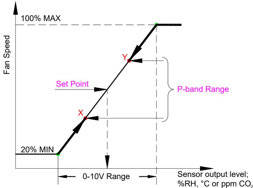
If, for example, the fan speeds are 20% and 100% (Note! Factory defaults are 20% and 80%), and the P-band range is equivalent to, say, X and Y, then point X becomes the 20% fan speed and point Y becomes 100%. It can be seen that if the P-band is set too narrowly, the fan speed response becomes coarse.
