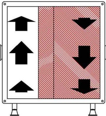
**DIRECTION OF AIRFLOW DISCHARGES OUT OF SHUTTER END**
