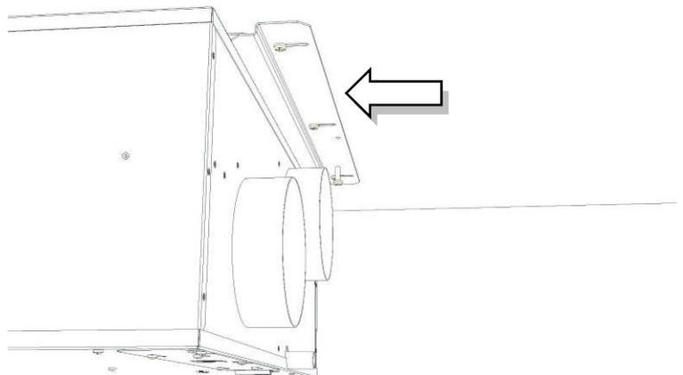
**Stage 4:** Finally, with the unit secure you can now fix the security fixing (as pictured right).
