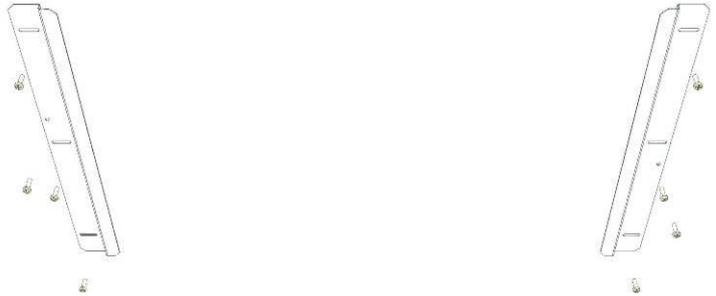
**Stage 2:** Place each of the bolts into position and **do not** fully tighten. Leave approximately “a half turn” loose on each of the fixings. This will allow each bracket to be moveable until final fitting of the unit and makes any adjustments easier while installing the unit in position.
