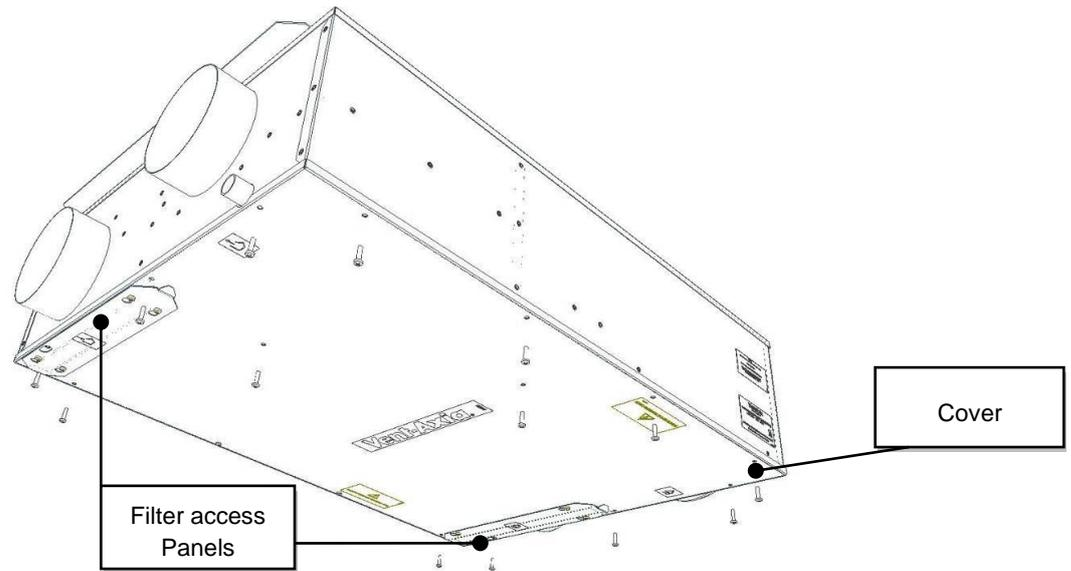
**Stage 1:** Isolate the mains power supply and remove the Filter access Panels and Filters.
