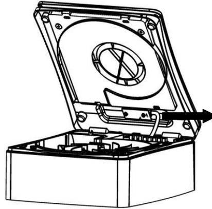
To remove the cover on TM models the sensor lead must be disconnected
