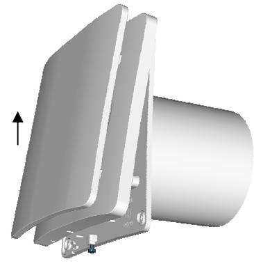
3. Push grille upwards until clear from the fan chassis.
