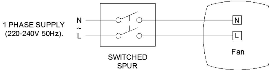
Fig.2 Continuous boost (15l/s) with no trickle facility
