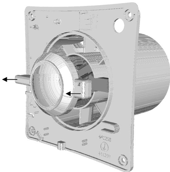
Fig.6. Removing the front grille panel for cleaning.
