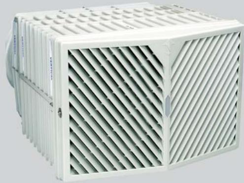
The HR500D is a self-contained unit with integral extract and supply fans to provide balanced ventilation and heat recovery via supply diffusers and extraction grilles. The unit is fully speed controllable.
